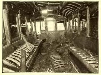
INTERIOR OF SECOND CAR AFTER FIRE, FIRE STARTED UNDER FLOOR
