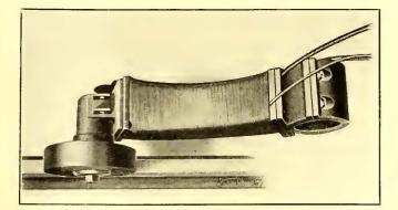
FIG. 2.--VIEW LOOKING DOWN ON MAGNETIC ADHESION ATTACHMENT
