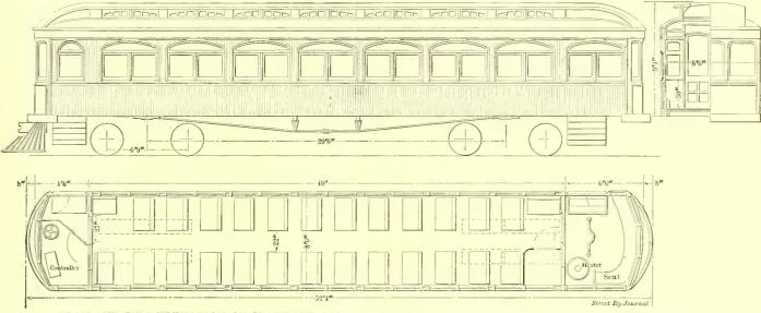
PLAN AND SIDE ELEVATION OF STANDARD CAR USED BY THE UNDIANA NORTHERN TRACTION COMPANY
