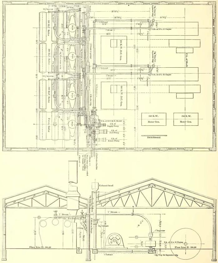
PLAN AND CROSS SECTION OF POWER STATION
