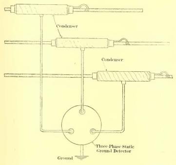
CONNECTIONS OF THREE-PHASE STATIC GROUND DETECTOR
