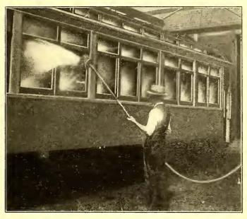
METAL CAR BRUSH, WITH ATTACHMENT FOR SPRAYING
