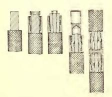
FIG. 1.—MANNER OF ASSEMBLING JOINT
