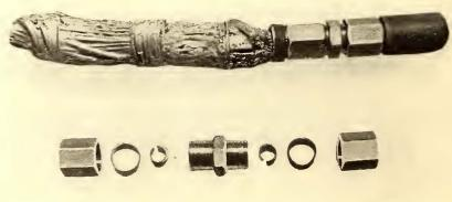
FIG. 6.—SHOWING SOLDERED JOINT AND NEW COUPLING, AND PARTS OF THE LATTER
