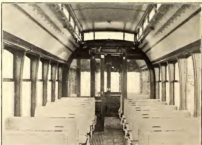
INTERIOR OF COMBINATION SEMI-CONVERTIBLE CAR FOR THE CALUMET ELECTRIC STREET RAILWAY COMPANY
