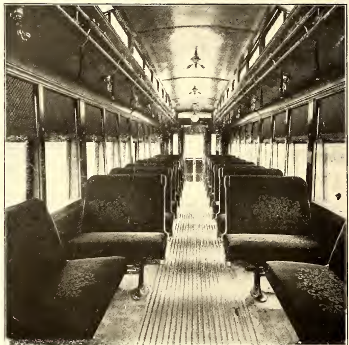
INTERIOR OF CAR FOR ATLANTIC SHORE LINE RAILWAY port, Maine, the type of car shown in accompanying illustrations. The car body is of the semi-convertible type, 35 ft. long over
