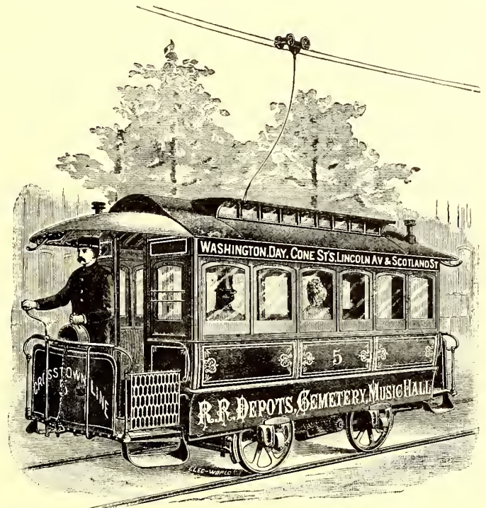
FIG. 6.—MOTOR CAR IN ORANGE, N. J., WITH MOTORS UNDER CAR
