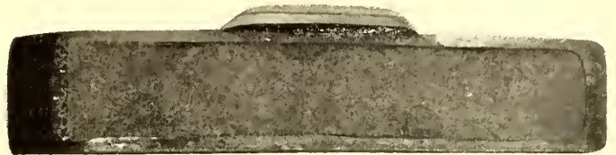
WOOL FELT FRICTION-PLATE FOR EMERGENCY CAR BRAKE
