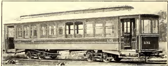
SEMI-CONVERTIBLE COMBINATION PASSENGER AND SMOKING CAR FOR THE CALUMET ELECTRIC STREET RAILWAY COMPANY
