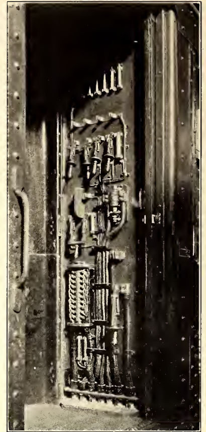
VIEWS OF THE MOTORMAN'S CONTROL APPARATUS AND THE CAR SWITCHBOARD LOCATED UPON THE PLATFORM
