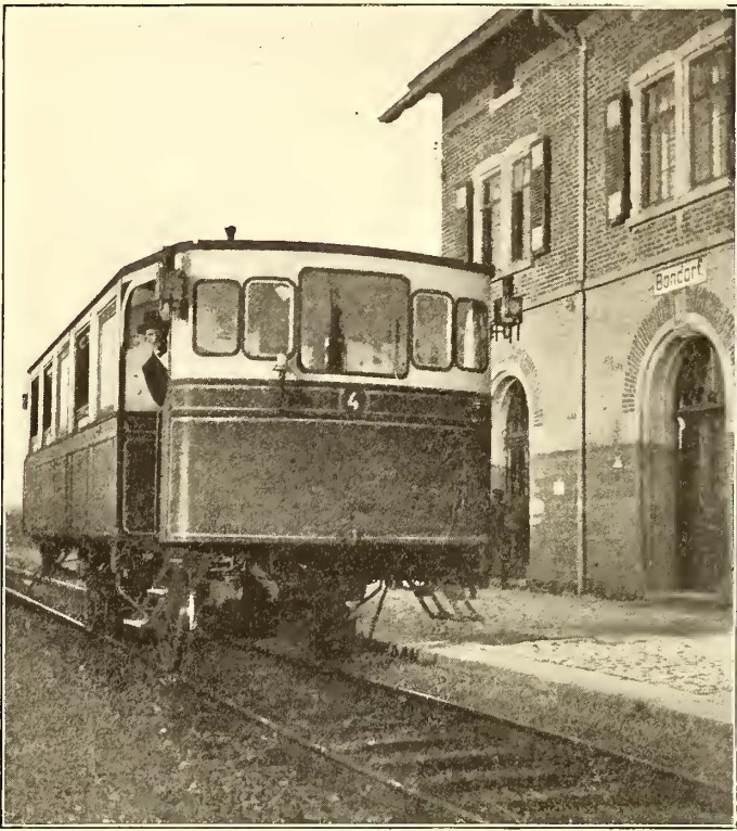
FIG. 10.—END VIEW OF PETROL MOTOR CAR USED BY THE WURTEMBERG STATE RAILWAYS
