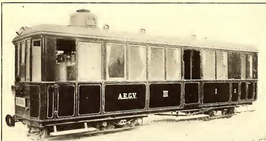
NARROW GAGE STEAM MOTOR CAR OF 35-HP CAPACITY USED ON THE ALFOLDER RAILWAY
