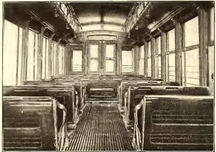
VIEW OF INTERIOR, SHOWING FRONT SEATS ARRANGED FOR SUMMER USE AND THE REAR SEATS ARRANGED FOR WINTER
