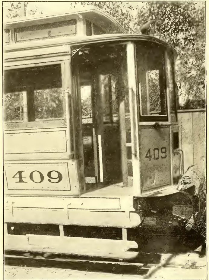
FIG. 5.—END VIEW, SHOWING SLIDING DOOR INSERTED INTO FRONT BULKHEAD AND PARTITION FOR MOTORMAN'S CAB
