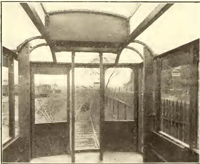
END VIEW OF ALL-STEEL CAR, SHOWING SPACE IN CORNER FOR SLIDING SIDE DOORS
