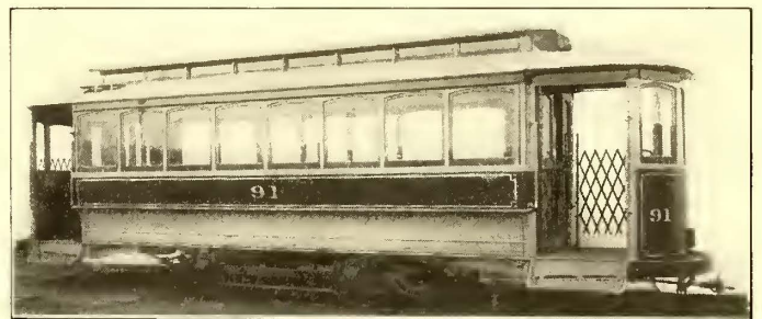
ONE OF THE SPRINGFIELD CONSOLIDATED COMPANY'S CARS FURNISHED WITH HIGH FOLDING GATES
