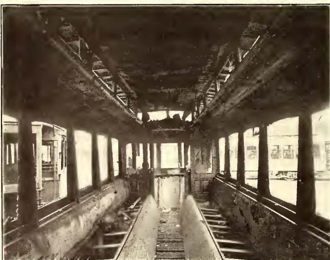
CAR IN TEST NO. 3—AFTER THE FIRE
