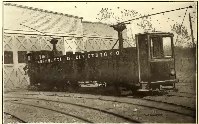
FIG. 22.—CINDER CAR USED FOR CONVEYING ASHES FROM THE POWER HOUSE
