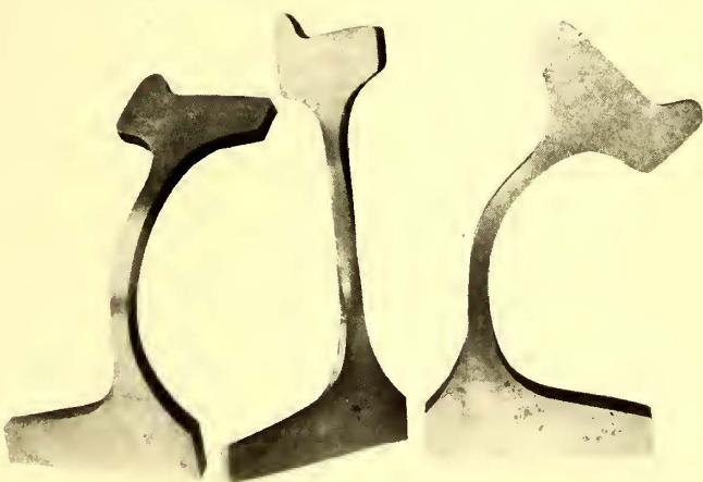
THIN RADIAL SECTIONS OF THE SOLID-STEEL WHEELS, SHOWING HOMOGENEITY AND REMARKABLE STRENGTH UNDER PHYSICAL TEST
