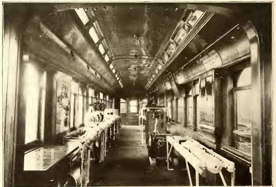
GENERAL INTERIOR VIEW OF THE BROOKLYN ELEVATED INSTRUCTION CAR, SHOWING THE OMISSION OF BODY END BULKHEADS
