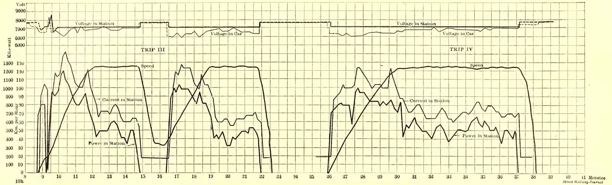
FIG. 13.—VOLTAGE, CURRENT, POWER AND SPEED CURVES FOR TRIPS III. AND IV.
