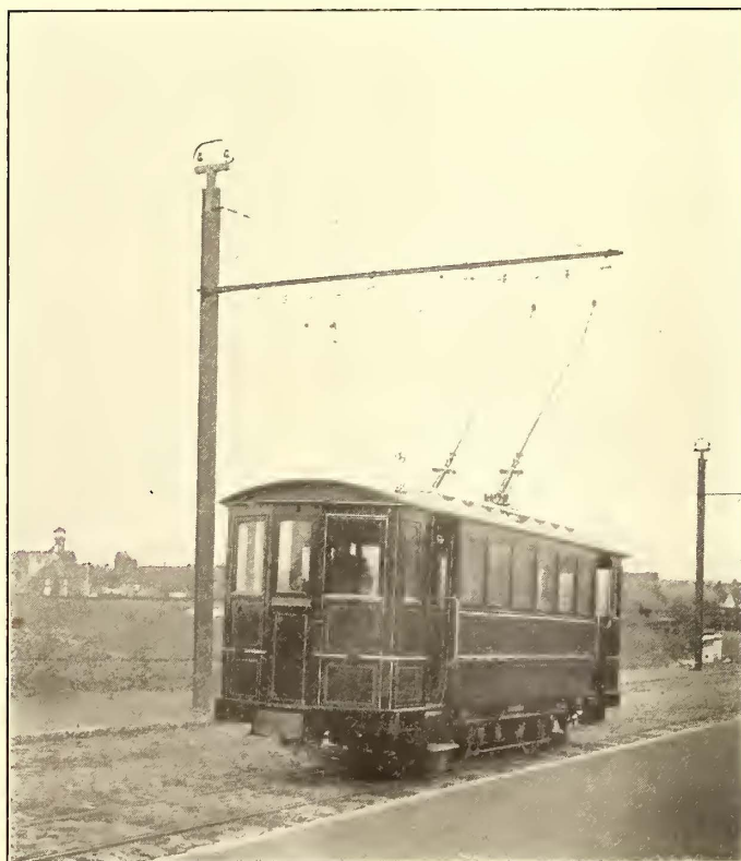
STANDARD MOTOR CAR USED ON THE BORINAGE SINGLE-PHASE RAILWAY SYSTEM
