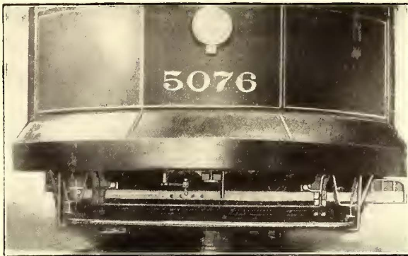
FIG. 9.—DISAPPEARING STEP (TAKEN FROM CAR-HOUSE PIT)
