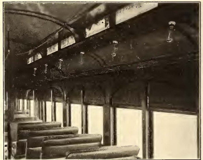
INTERIOR OF STANDARD CAR, SHOWING THE TYPES OF SEATS AND WINDOWS, LIGHTING ARRANGEMENT, ETC.
