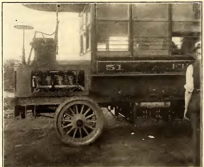
FIG. 6.—SIDE VIEW, SHOWING LOCATION OF GASOLINE MACHINERY UNDER DRIVER'S SEAT
