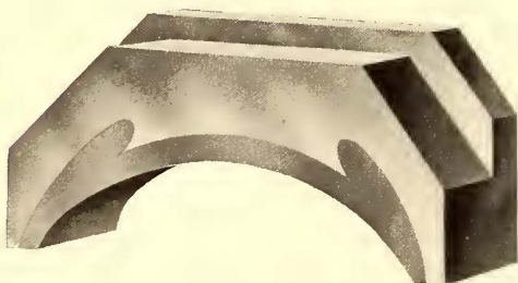
FIG. 1.—BRONZE SHELL FOR JOURNAL BEARING
