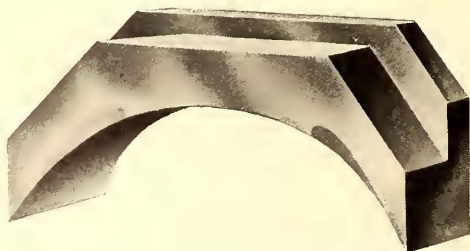
FIG. 3.—SECTIONAL VIEW OF CAR JOURNAL BEARING AFTER RUNNING 72,000 MILES
