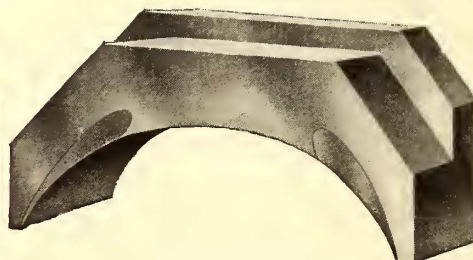
FIG. 2.—SHOWING BABBITT WORN TO LINE OF BRONZE
