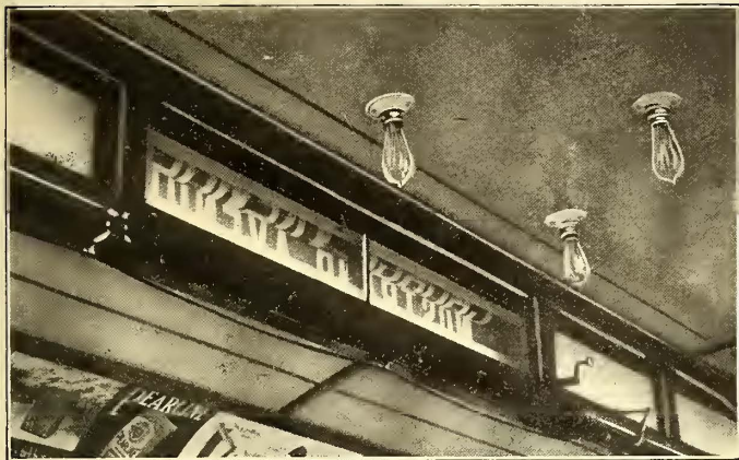
FIG. 20.—SIGN, SHOWING POSITION OF LAMPS BEHIND IT
