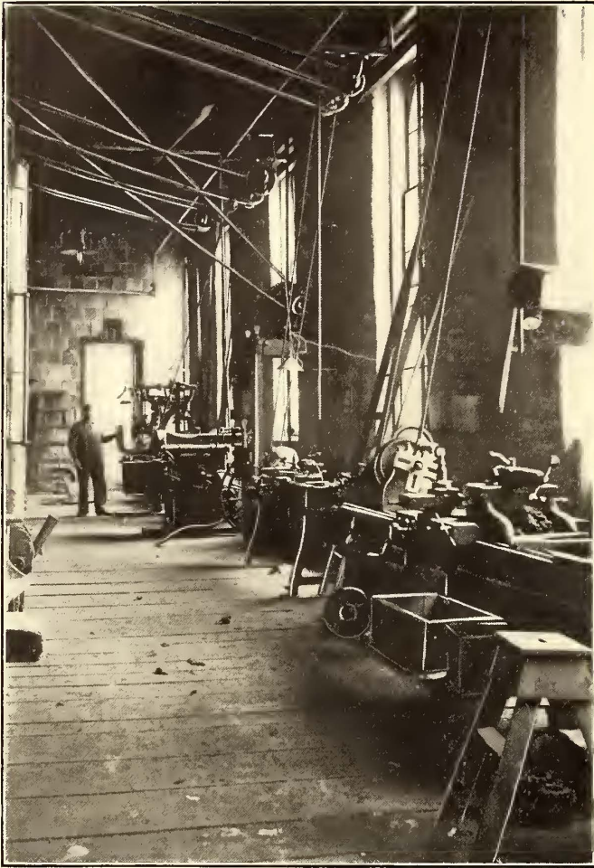
FIG. 1.—MACHINE TOOLS DRIVEN BY ONE MOTOR
