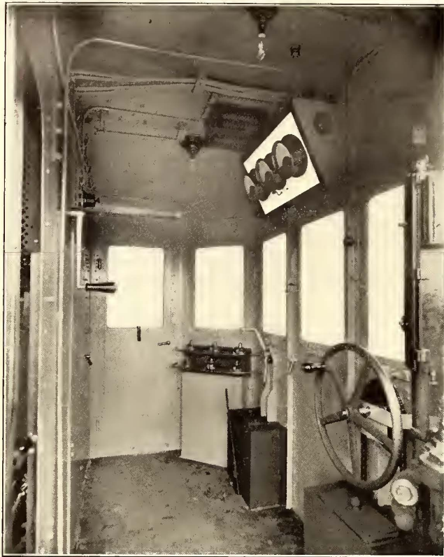
MOTORMAN'S CAB OF 15,000-VOLT, SINGLE-PHASE LOCOMOTIVE
