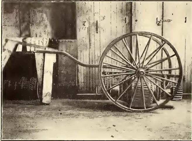
FIG. 5.—AN ARMATURE CART WHICH ELIMINATES HEAVY LIFTING
