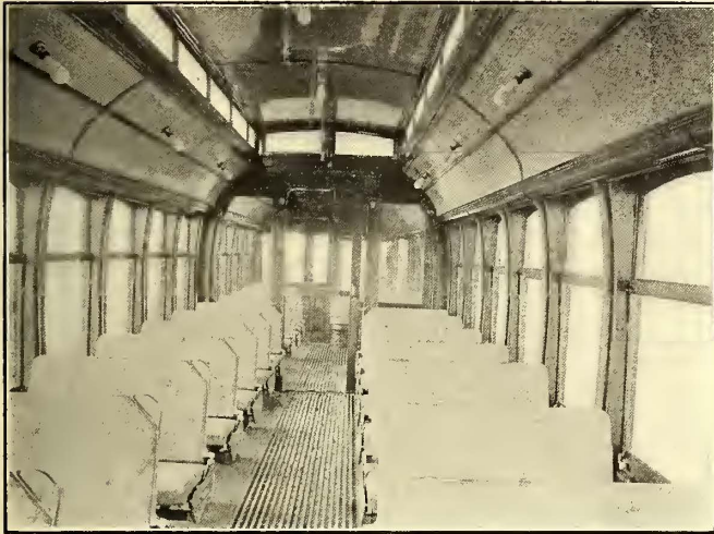
INTERIOR VIEW OF LEXINGTON CAR, SHOWING SEATING AND LIGHTING ARRANGEMENT
