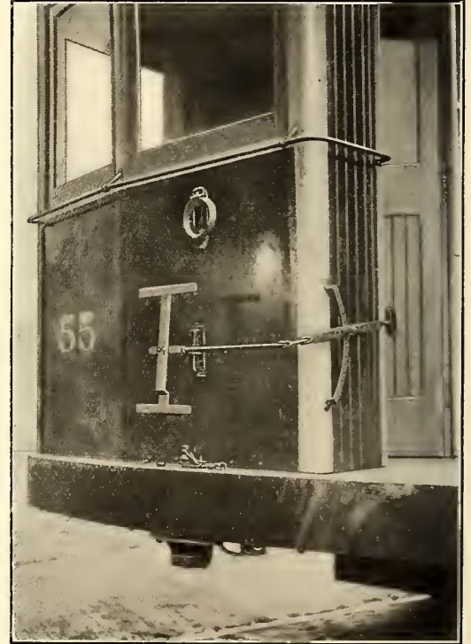
FIG. 8.—ADJUSTABLE HEADLIGHT BRACKET FOR LINE CAR
