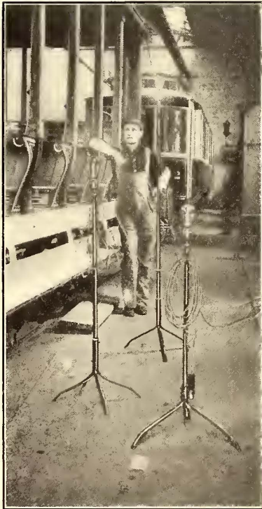
FIG. 6.—ADJUSTABLE LAMP STANDS FOR USE IN THE PAINT SHOP
