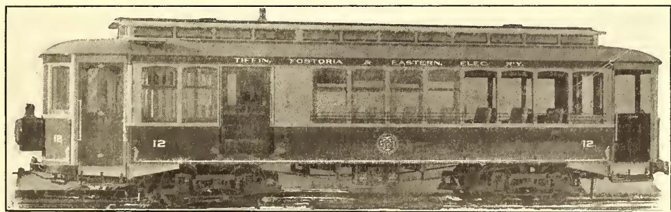
COMBINATION PASSENGER AND BAGGAGE CAR FOR THE TIFFIN, FOSTORIA & EASTERN ELECTRIC RAILWAY
