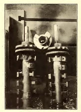
FIG. 4.—A BURNED CONTROLLER AND A REPAIRED ONE, WITH REPAIR CASTING
