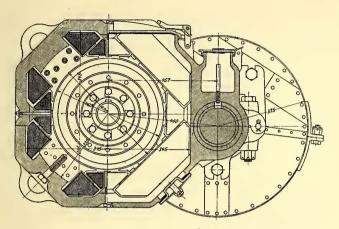
CROSS SECTION OF INTER-POLE RAILWAY MOTOR
