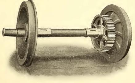
STANDARD WHEEL, AXLE, AND GEAR, AND SPECIAL MOTOR AXLE BEARING WITH COLLAR USED AT BIRMINGHAM
