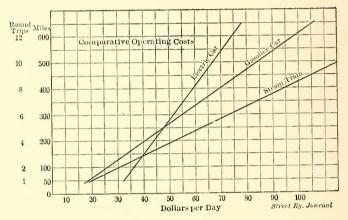
FIG. 2.—CURVES SHOWING COMPARATIVE OPERATING COST OF THREE SYSTEMS OF TRACTION, RUNNING STATED NUMBER OF TRIPS PER DAY
