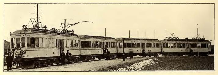
A TRAIN OF TWO MOTOR CARS AND TWO TRAILERS ON THE 990-VOLT DIRECT-CURRENT LINE BETWEEN COLOGNE AND BONN
