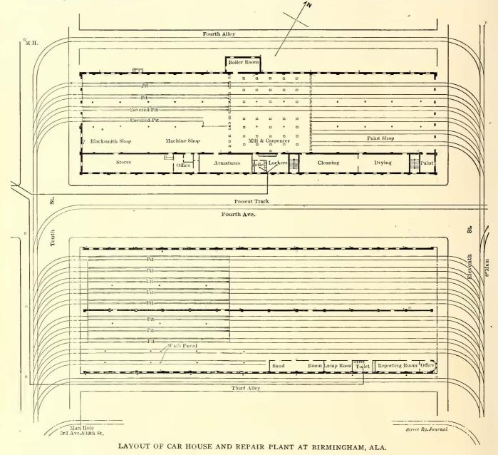
ter mechanic and assistant superintendent. J. L. Mason is assistant master mechanic. The plant consists of two independent buildings, separated by an 80-ft. street.
