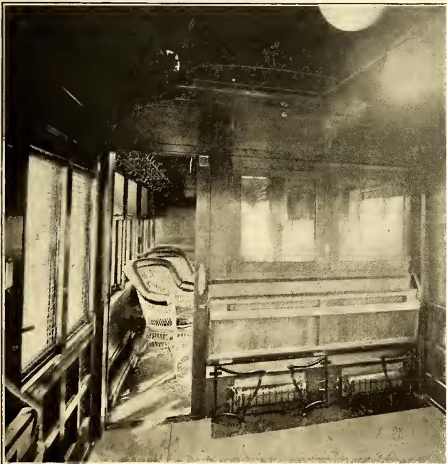
BAGGAGE COMPARTMENT, SHOWING FOLDING SEAT, HEATERS AND SMOKING ROOM BEYOND
