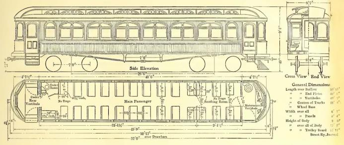
ELEVATION, END VIEW AND PLAN OF LIMITED SERVICE CAR FOR THE LAKE SHORE ELECTRIC RAILWAY
