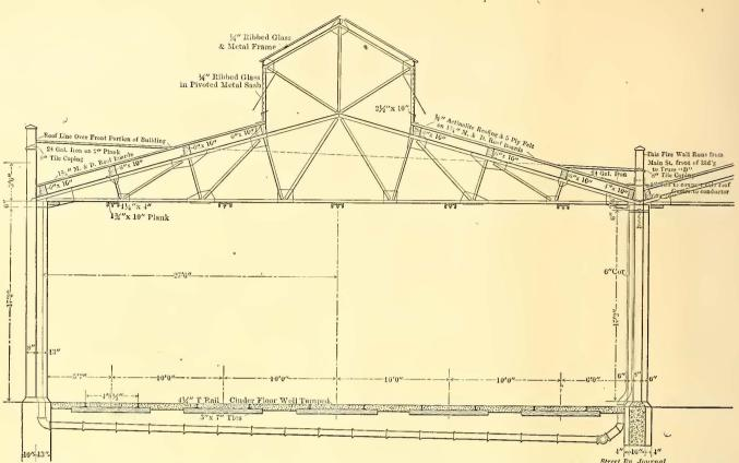
CROSS-SECTION OF CAR HOUSE ALONG THE LINE B-B ON PLAN, SHOWING DETAILS OF FLOORING, WALLS AND ROOF CONSTRUCTION
