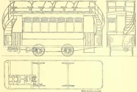
ELEVATIONS AND PLAN OF GASOLINE STREET CAR
