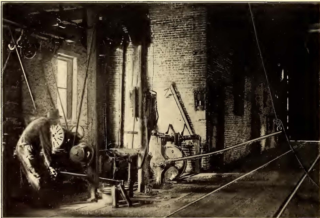
FIG. 1.—DEVICE FOR APPLYING POWER TO A HAND-OPERATED WHEEL PRESS
