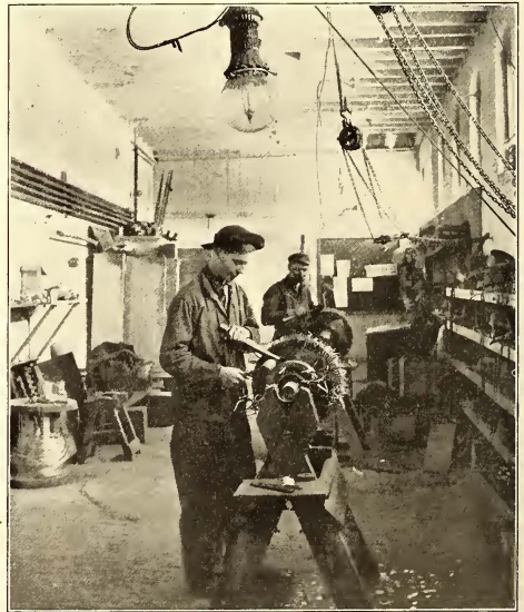
IN THE ARMATURE-WINDING ROOM
