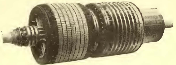
ROTOR WINDINGS OF MOTOR CONVERTER
