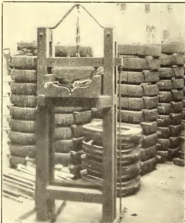
PRESS FOR SHAPING COILS; ALSO SHOWING THE MANNER OF STORING THEM
