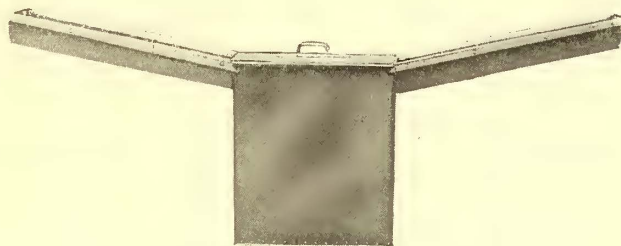
DRIP CAN WITH EXTENDING SPOUTS USED IN THE WINDING ROOM
