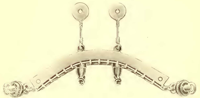
THE GUARD AS INSTALLED TO PROTECT DOUBLE TROLLEY
