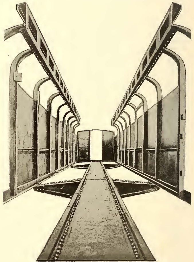
UNDERFRAME AND SIDE POSTS OF PENNSYLVANIA STEEL MAIL CAR, SHOWING TYPE OF CENTER SILL AND CROSS BEARERS USED IN PASSENGER COACH
