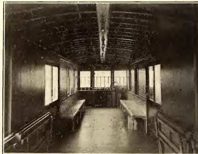
INTERIOR OF BOISE FREIGHT CAR, SHOWING SEATS ADAPTED TO THE USE OF MINERS
