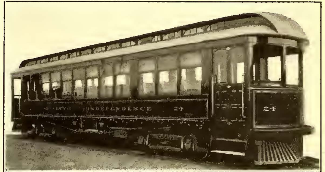
INTERURBAN SEMI-CONVERTIBLE CAR FOR THE SERVICE BETWEEN INDEPENDENCE AND CHERRYVALE, KANSAS
