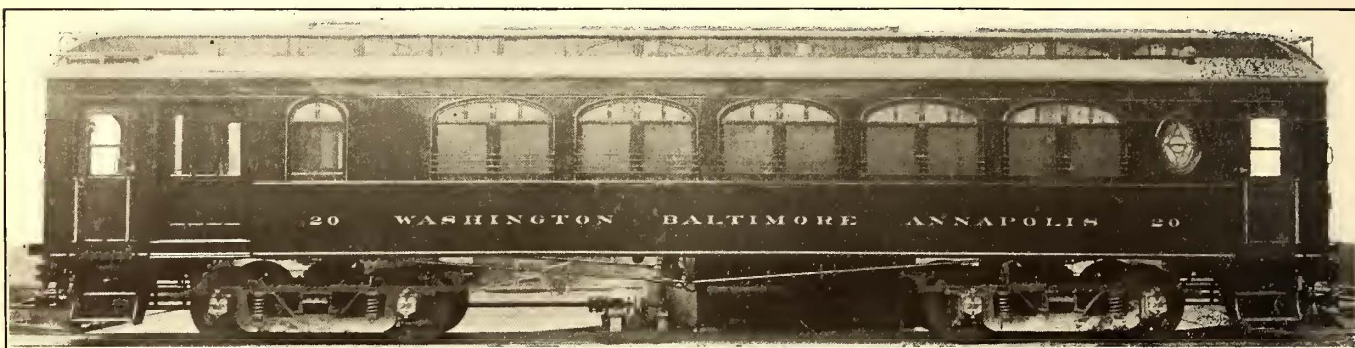
COMBINATION CAR FOR THE WASHINGTON, BALTIMORE & ANNAPOLIS ELECTRIC RAILWAY
