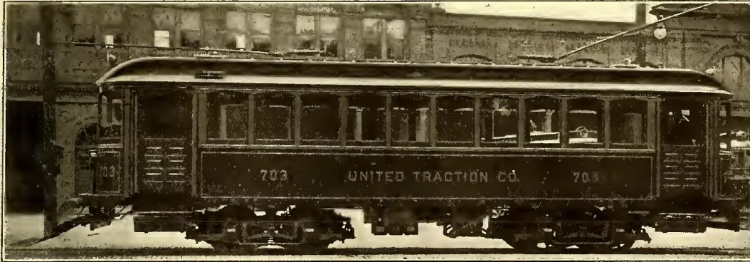
APPEARANCE OF THE NEW TROY CAR WHEN THE DOORS ARE CLOSED AND THE STEPS ARE UP
