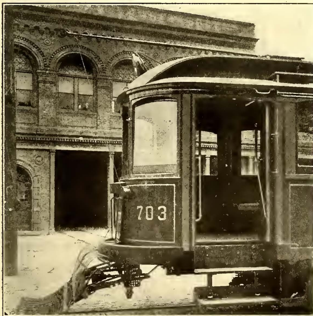
VIEW OF THE TROY CAR WITH THE DOOR OPEN AND THE STEPS DOWN. THE GRAB HANDLES ARE INSIDE THE CLOSED DOOR
