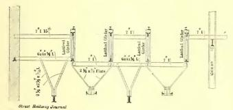
SECTION, SHOWING METHOD OF ATTACHING CHAIN-HOIST CHANNELS AND CONDUCTOR ANGLES TO SECOND-FLOOR GIRDERS
