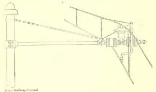
FIG. 1.—BRACKET CONSTRUCTION FOR CURVES
