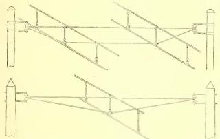
FIG. 5.—MODIFICATION OF CROSS-SPAN CONSTRUCTION WITH SINGLE INSULATOR
