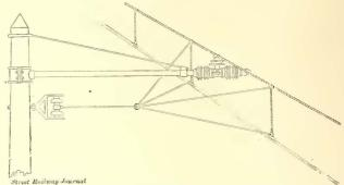
FIG. 3.—AUXILIARY INSULATORS AND PYRAMIDAL GUYING TO YOKE INSULATOR
