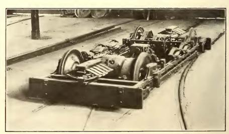
END VIEW OF TRUCK, SHOWING METHOD OF MOUNTING MOTORS AND AIR COMPRESSOR ON TRUCK; ALSO ARRANGEMENT OF SPRINGS
