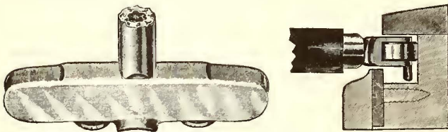
VIEWS OF THE CURTAIN FIXTURES, SHOWING THE FLANGE AND THE APPLICATION OF THE CONFINING STRIP
