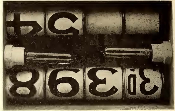
BACK OF BOX, SHOWING ROLLS AND LAMPS
