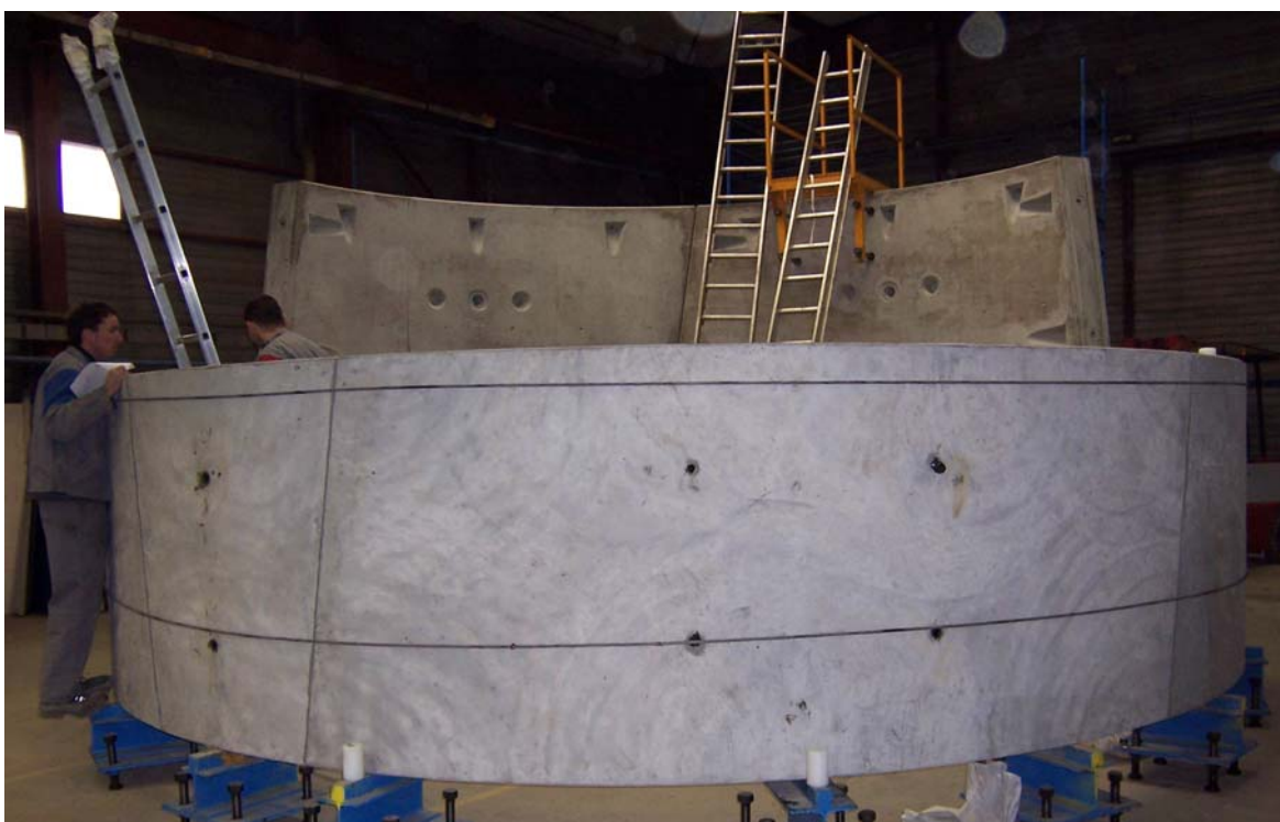
Demonstration test of tunnel liners in Tours, France.
