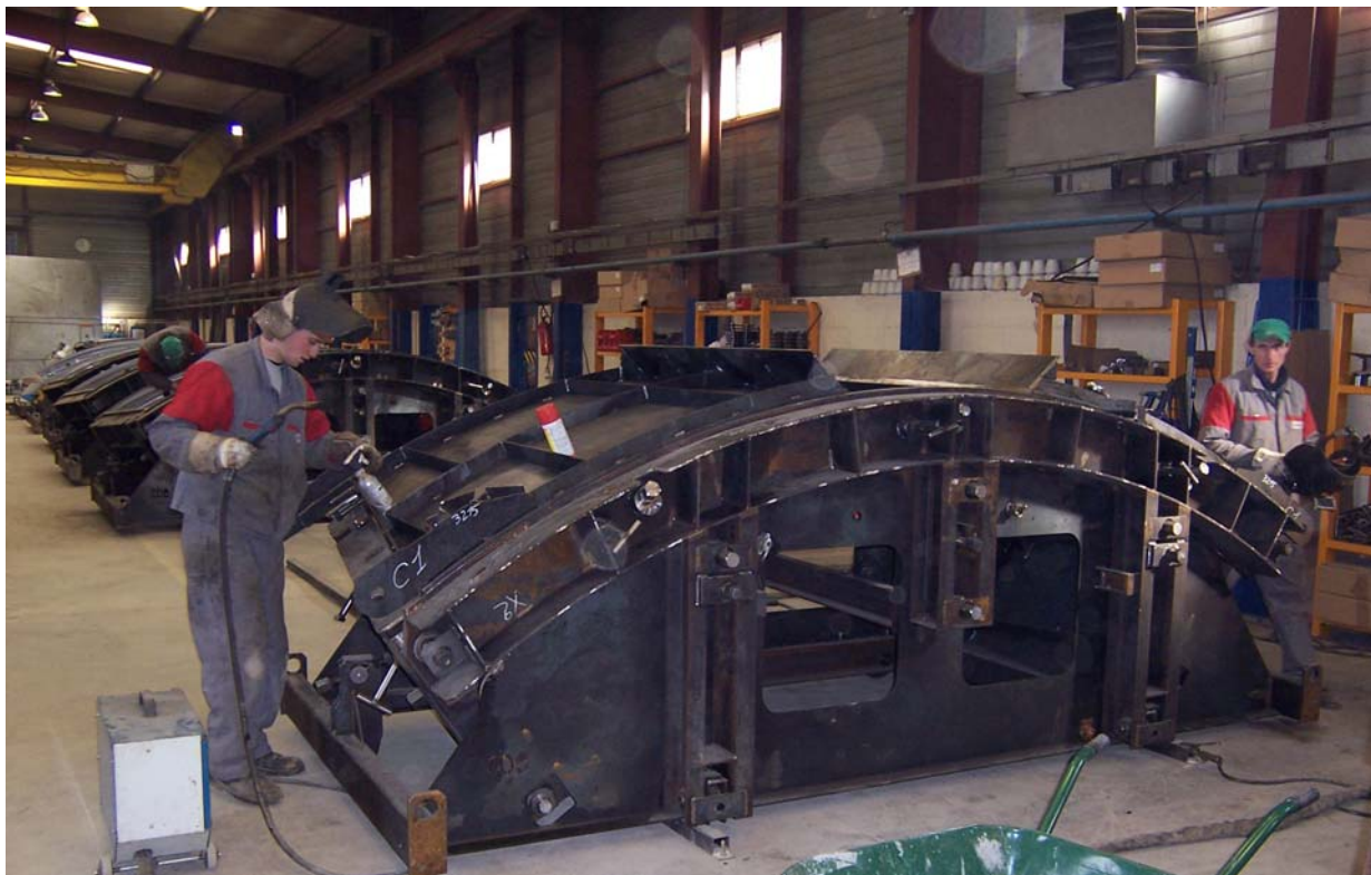
Fabrication of tunnel liner molds in Tours, France.
