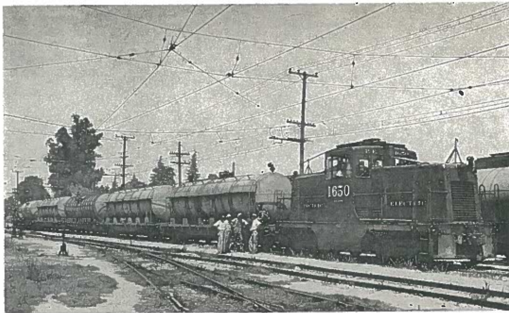
FREIGHT BEING MOVED BY 44-TON 380-HP DIESEL ELECTRIC LOCOMOTIVE Trolley Actuates Wigwag Signals at Highway Crossings
