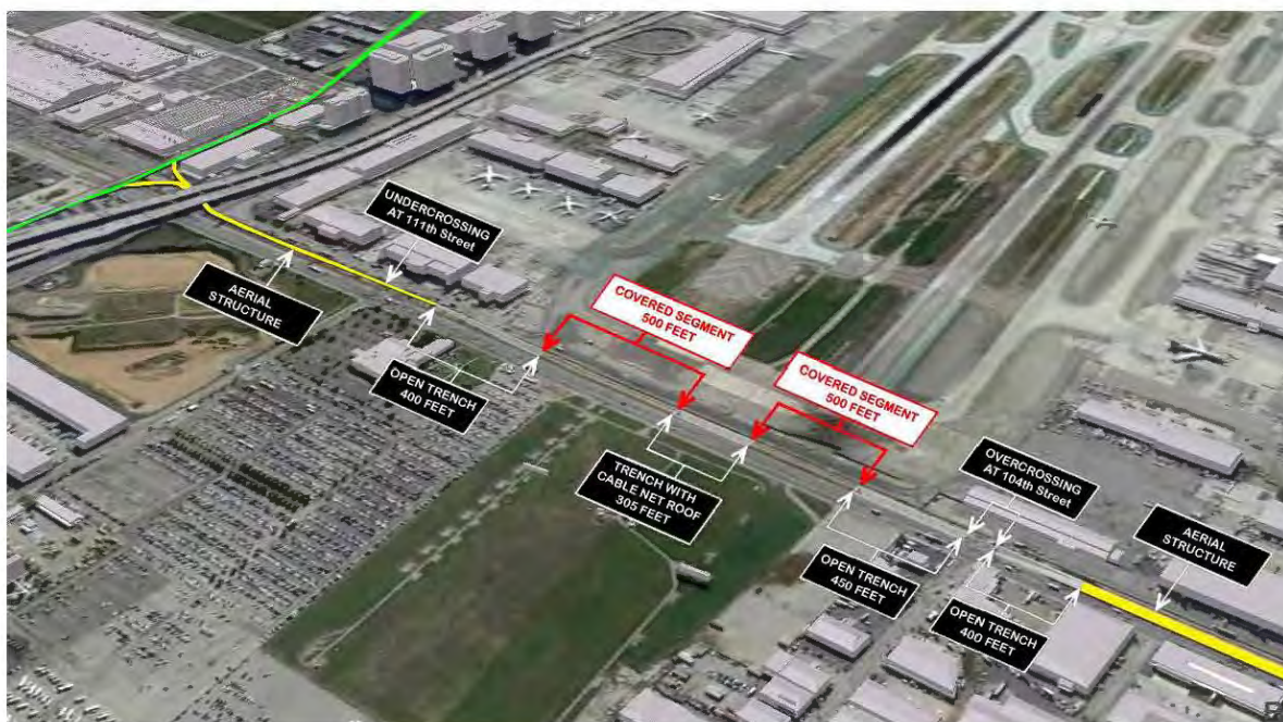
The Partially-Covered LAX Trench Option (interim solution) would be covered directly in front of the runways and have open sections in the middle and on the ends.
