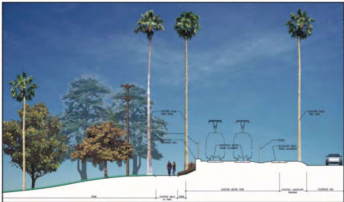
Cross-section view of LRT alignment along Harbor Subdivision adjacent to Edward Vincent Jr. Park and Florence Avenue showing that the majority of palm trees would be retained resulting in no adverse visual effects.
