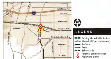
Design Option 6 is a below grade alignment along Crenshaw Boulevard between Exposition and 39th Street.
