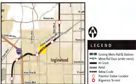
Design Option 3 is a grade separation at the Harbor Subdivision and Centinela Avenue.
