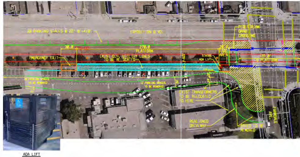
Figure 3a: Proposed LRT Passenger Station Plan with At-grade Crossing – Eastbound Platform, West of Farmdale Avenue
