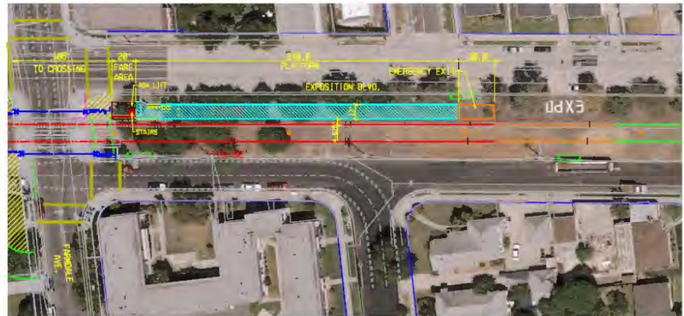
Figure 3b: Proposed LRT Passenger Station Plan with At-grade Crossing – Westbound Platform, East of Farmdale Avenue
