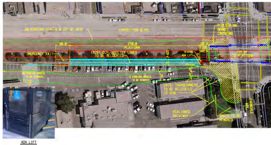
Figure 3a: Proposed LRT Passenger Station with At-grade Crossing – Eastbound Platform West of Farmdale Avenue
