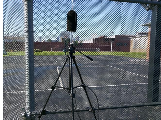
Figure B-6. Monitoring Location 1b Noise Meter, #1
