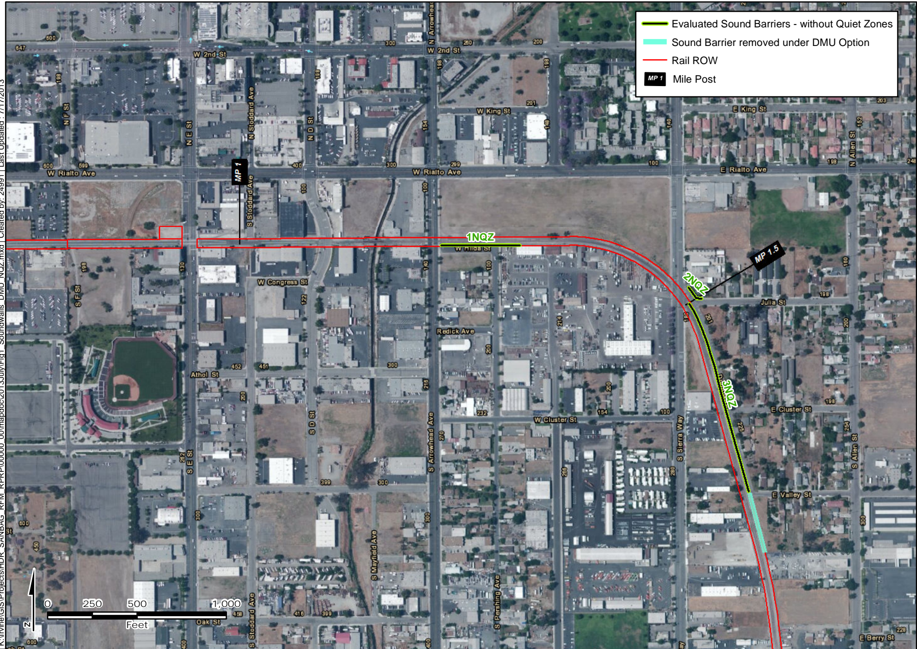
Evaluated Sound Barrier Locations Under DMU Option - Scenario without Implementation of Quiet Zones
