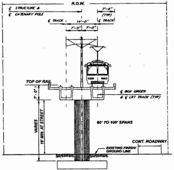
NOTE: CATENARY AND PANTOGRAPH SYSTEM APPLIES TO ALTERNATIVES 6 AND 11. ALTERNATIVES 1, 2, AND 11 COULD ALSO TAKE POWER FROM THIRD RAIL ON AERIAL SECTIONS
