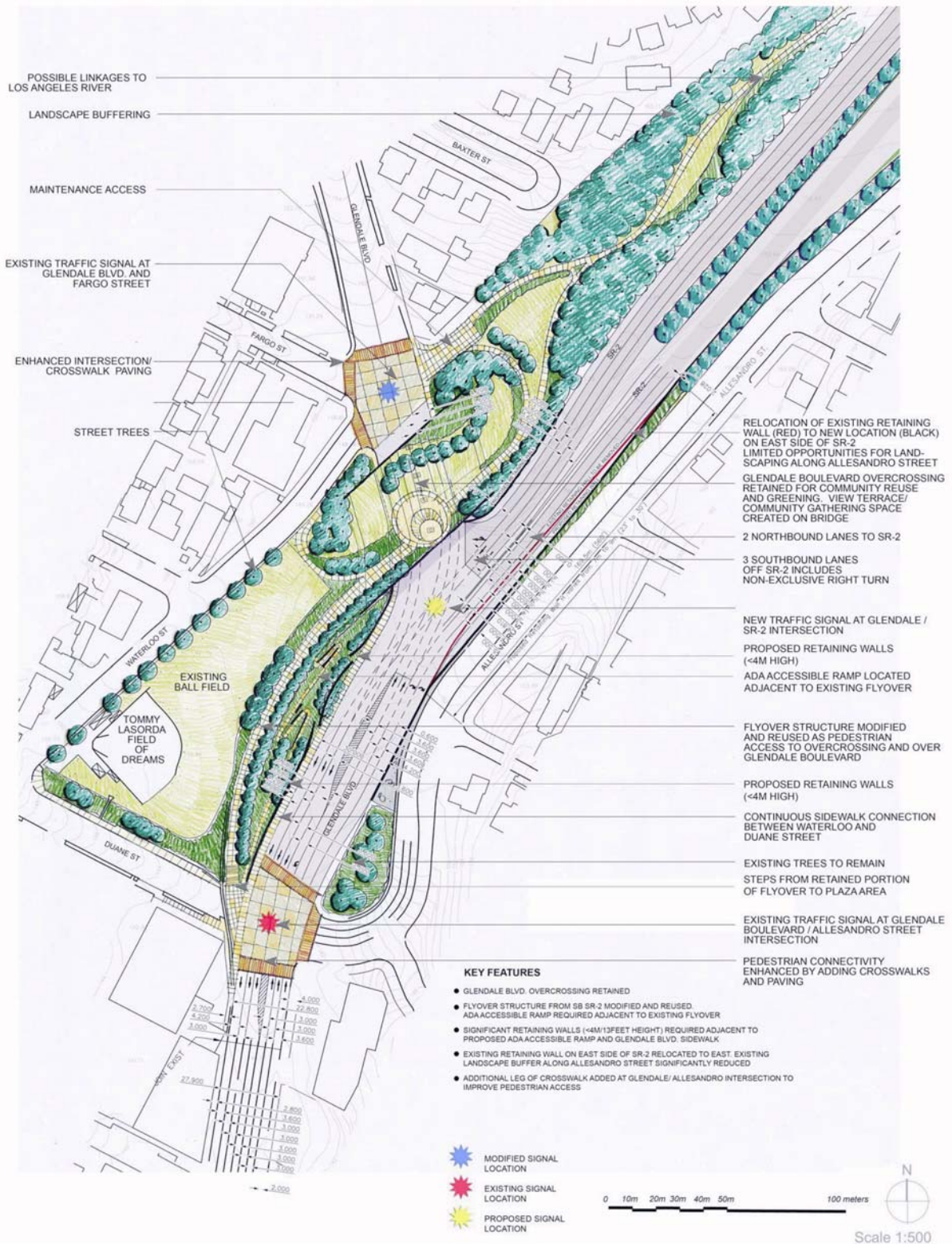
Figure 1-9. Alternative E (Realign Ramps East – Retain Flyover and Overpass – Relocate Retaining Wall)
