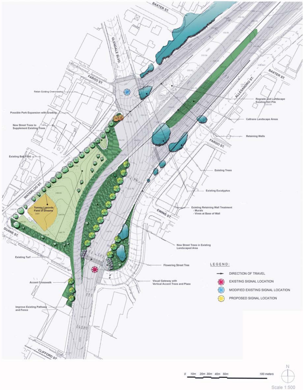
Figure 1-5. Alternative A (Widen Existing Ramps)
