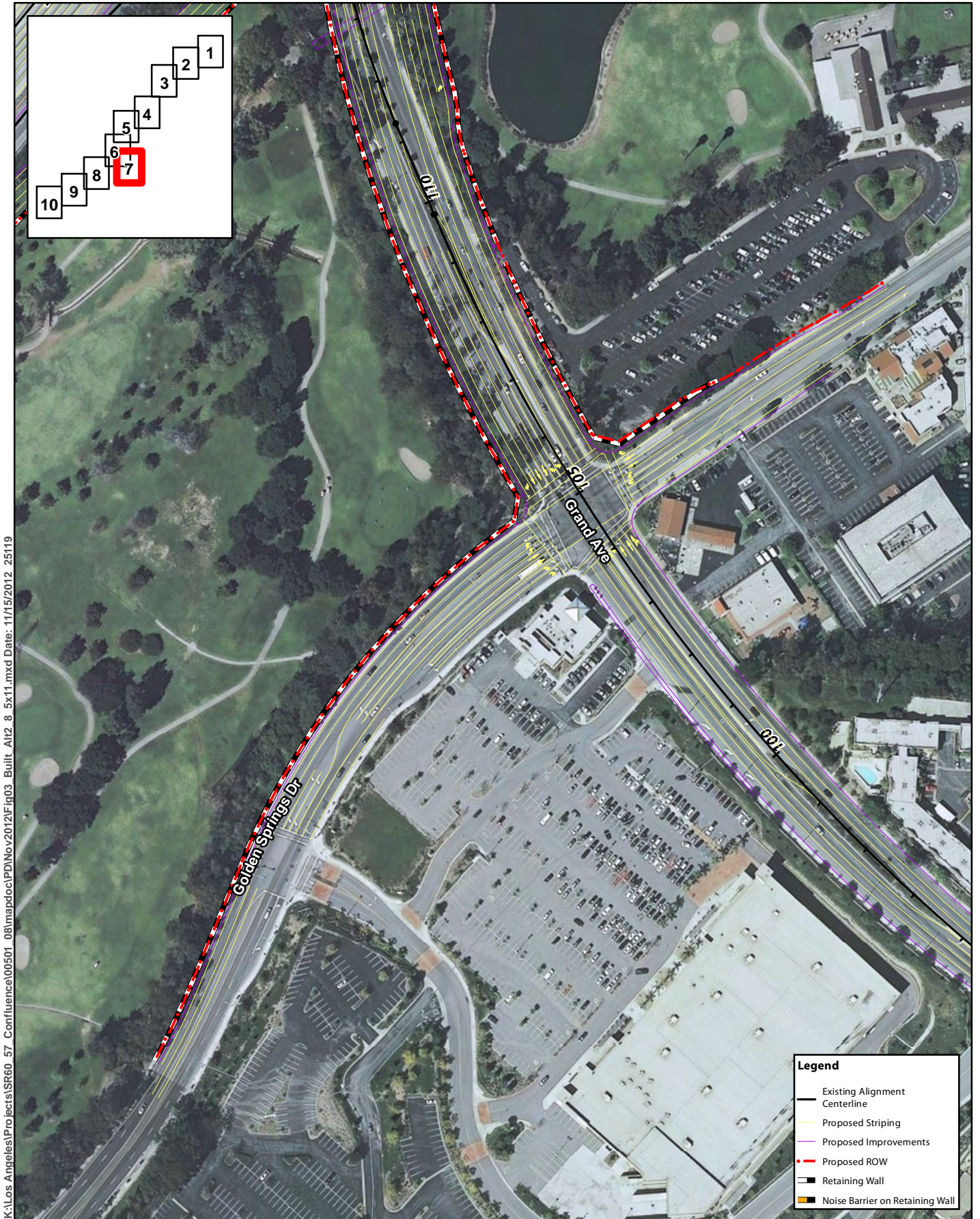
Figure 1-3- Sheet 7 of 10 Alternative 2, Combination Cloverleaf / Diamond Interchange Configuration State Route 57/State Route 60 Confluence at Grand Avenue Project
