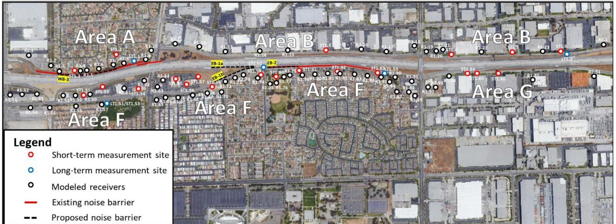
Figure 2.13-2. Analysis Areas, Noise Monitoring Positions, and Location of Evaluated Noise Barrier (Western Most Terminus)
