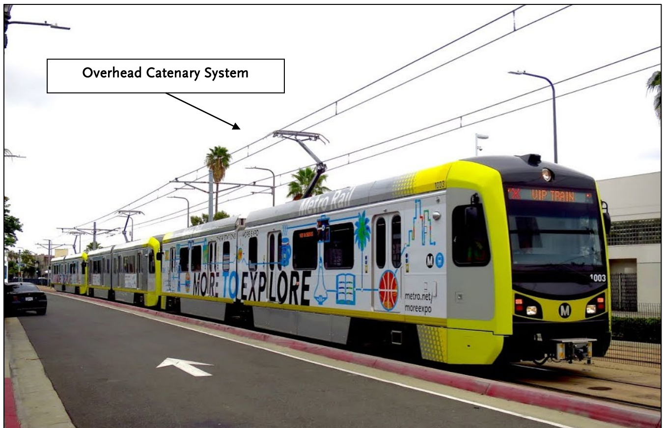
Figure 2.9 Metro Overhead Catenary System for Light Rail Transit Vehicles
