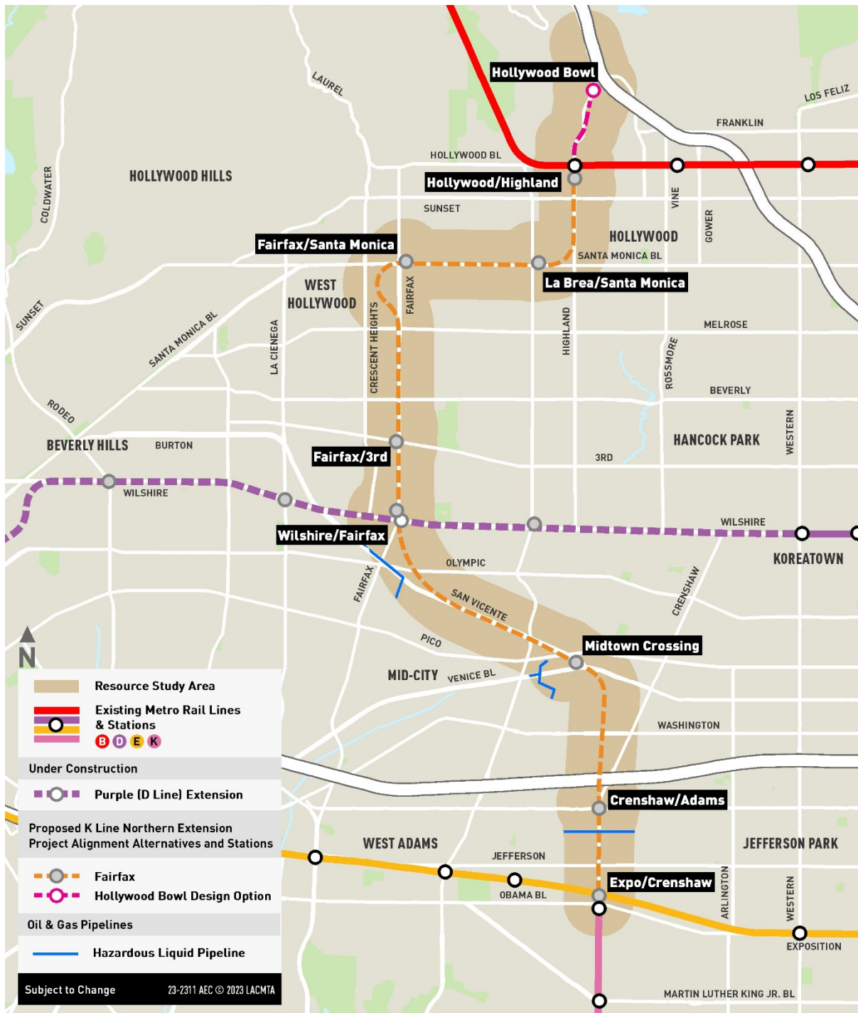
FIGURE 5-26. PETROLEUM PIPELINES ALONG FAIRFAX ALIGNMENT ALTERNATIVE
