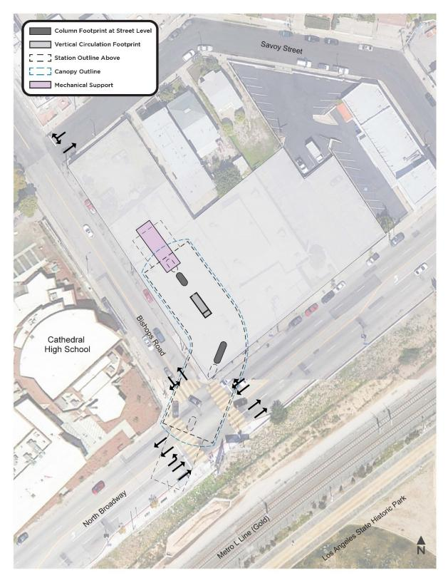
Figure 2-30: Broadway Junction Buildout Conditions
