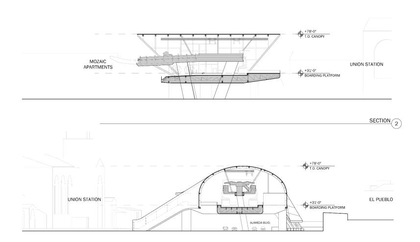
Figure 2-11: Alameda Station Cross Sections
