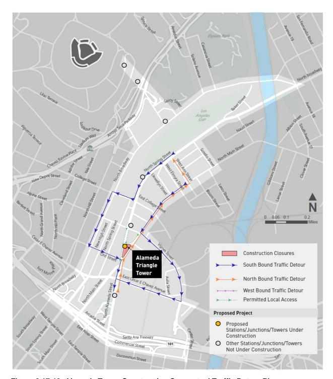
Figure 3.17-10: Alameda Tower Construction Conceptual Traffic Detour Plan
