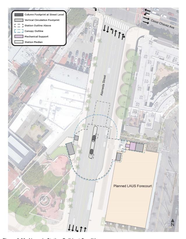
Figure 2-26: Alameda Station Buildout Conditions
