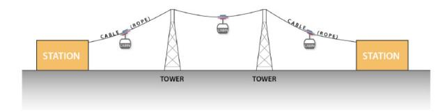
Figure 2-1: Aerial System Key Components
