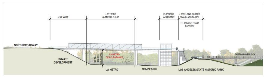
Figure 6-21: Design and Use Option E Section View (Bridge Feasibility Study Option 1)
