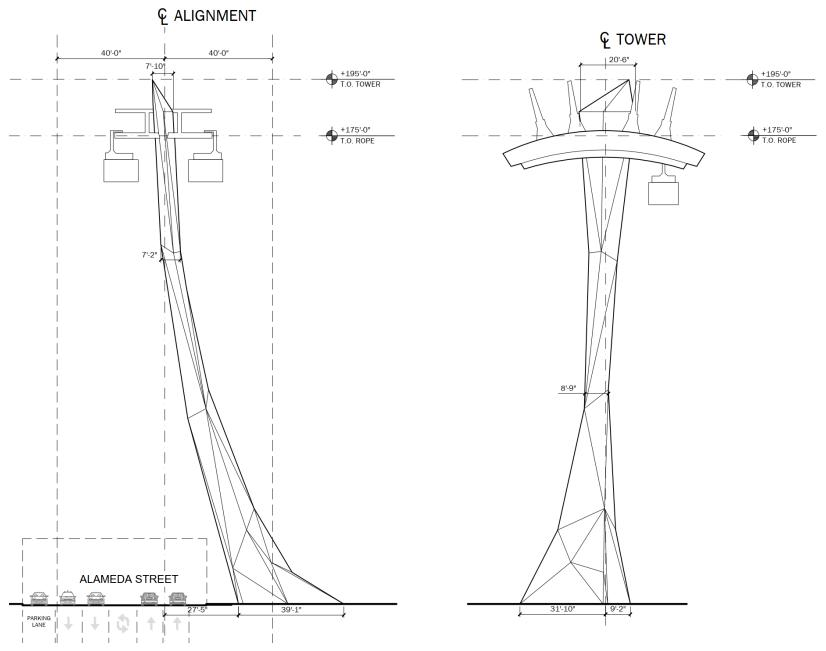
Figure 2-13: Alameda Tower Elevations
