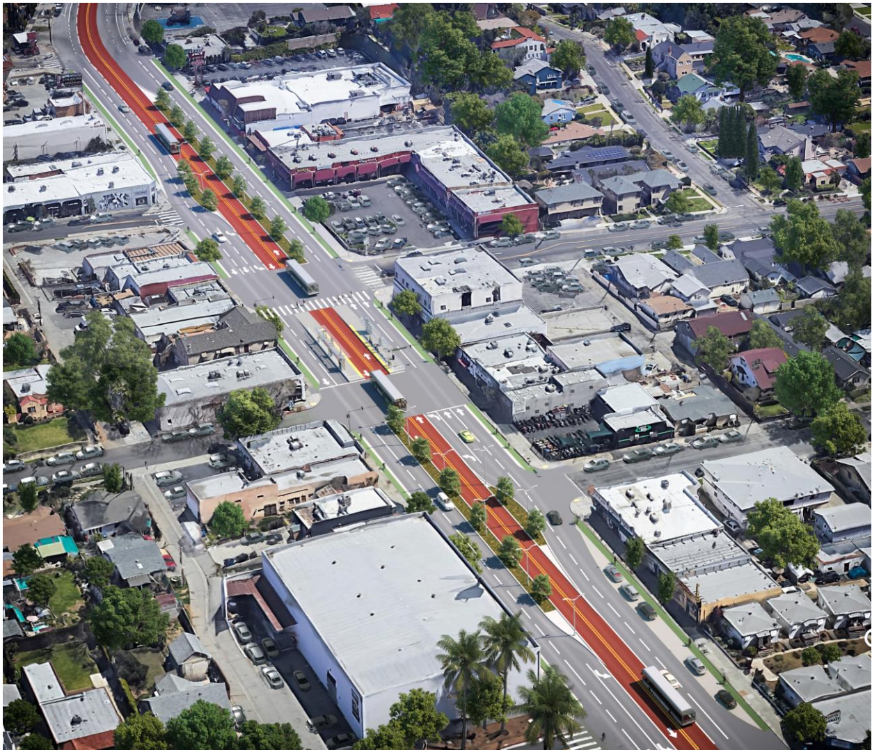
Figure ES-12 – Eagle Rock – Colorado Boulevard Post-Project (Design Option with Two Travel Lanes per Direction)
