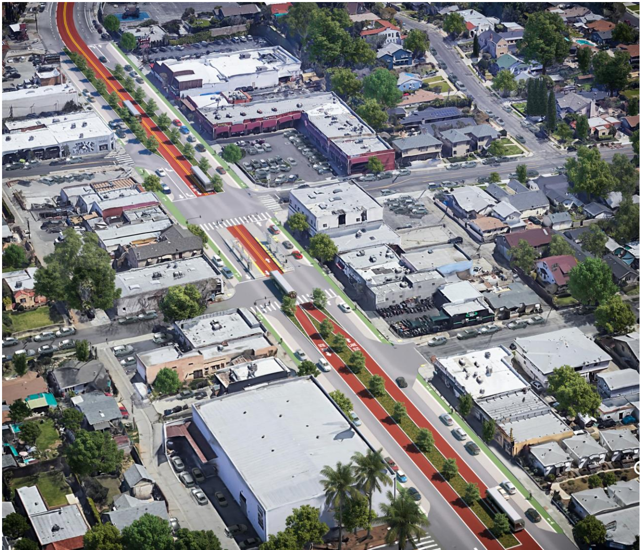
Figure ES-13 – Eagle Rock – Colorado Boulevard Post-Project (Design Option with One Travel Lane per Direction)
